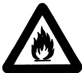
Flammable material or high temperature (1)
